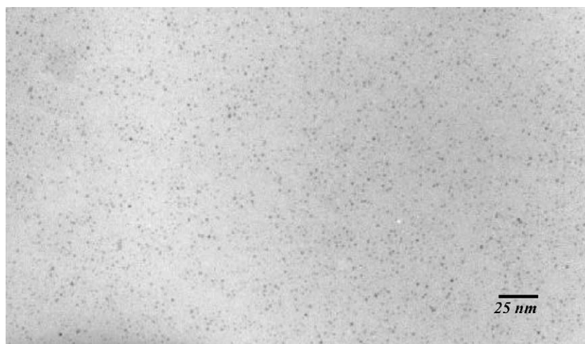
Fig. 1. TEM micrograph of Ru colloidal particles (COL-RU1).
